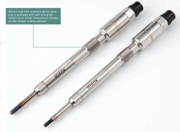
extremely high accuracy levels and real time measurement of pressure during the combustion process. The pressure information, amplified, calibrated and filtered by exclusive integrated ASIC is transmitted to the ECU to enable engine closed loop control, thus bringing improved fuel burn levels and reduced engine out emissions.
